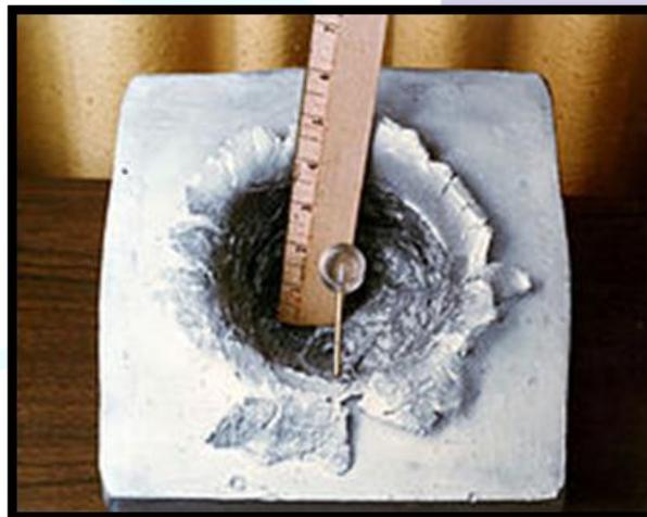
Figure 2: A 7 gram object (shown in centre) shot at 7 km/s (23,000 ft/sec) (the orbital velocity of the ISS) made this 15 cm (5 7/8 in) crater in a solid block of aluminium.<sup>11</sup>
