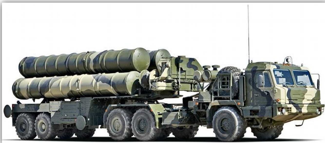
Image 1: S-400 Triumph (SA-21 Growler) Long Range Surface to Air Missile loaded on the Almaz TEL (Transporter Erector Launcher) towed by a 6x6 BAZ vehicle.
